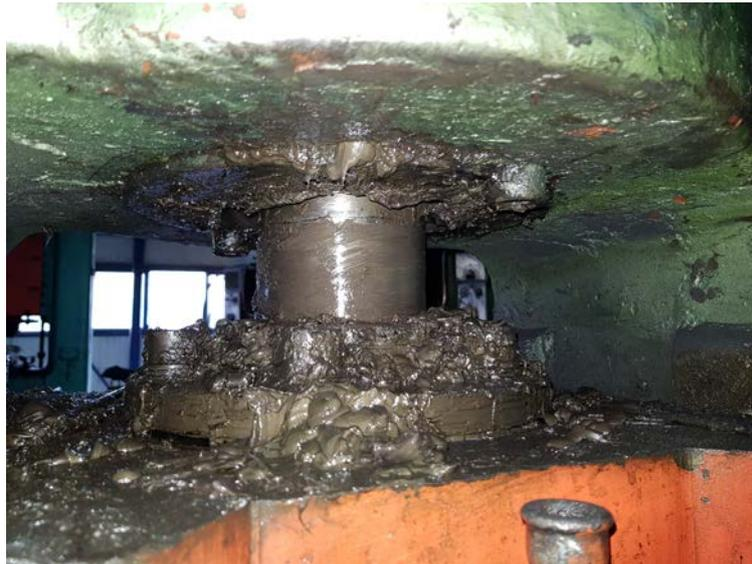
*Picture 4. – Repair of threaded spindle in exploitation*
