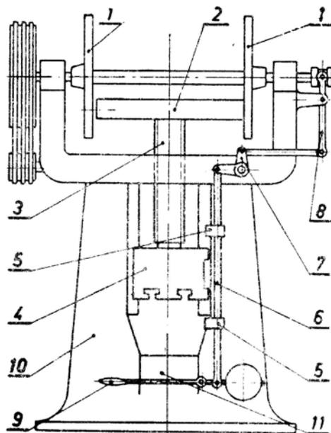
Picture 1. – Friction screw press [2]
