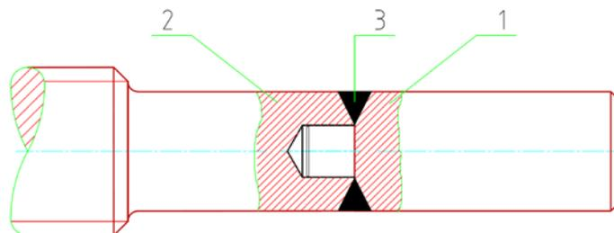
(c) - Velded joint: 1 - Threaded spindle extension, 2 - Healthy part of the threaded spindle, 3 - Weld
