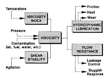
Limits for changes in the viscosity depend on the type of lubricant being analyzed but most often have a marginal limit of approximately 10% and a critical limit of approximately 20% higher or lower than the intended viscosity.
