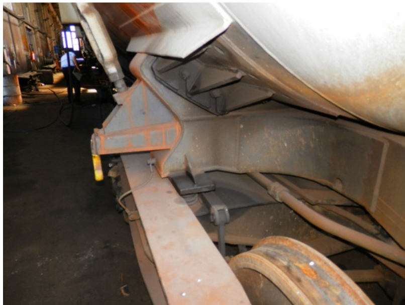
Picture 8. – The leakage point of the test fluid from the outside
