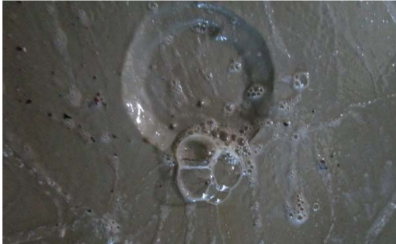
Picture 9. – The leakage point of the test fluid from the inside
